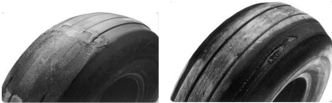
Figure 4: Shoulder wear (Source: Michelin and Goodyear)
