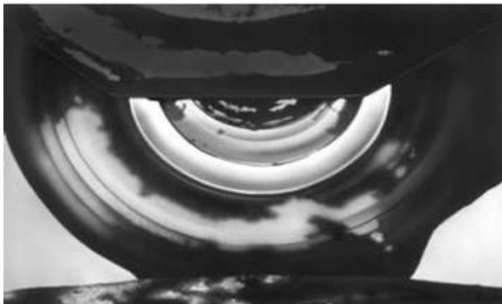
Figure 1 Traction wave in the tread surface (Source: Michelin and Goodyear)
